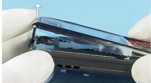
Lift the topside of the A-cover and then remove it carefully.
