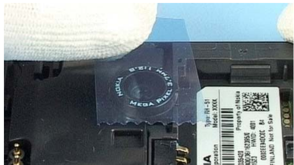
Protect the camera window with a film.
