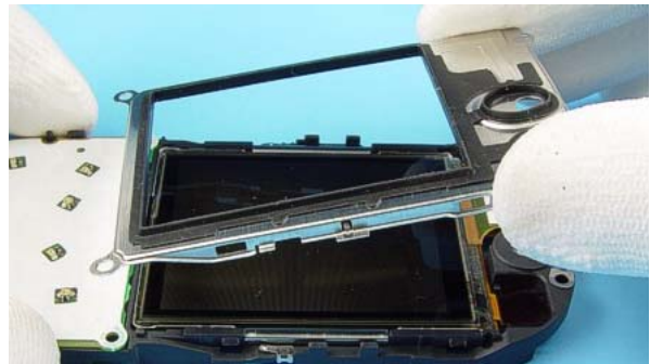
Now, the LCD top shield assy can be removed.
