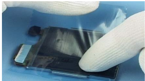
Protect the LCD module with a film.
