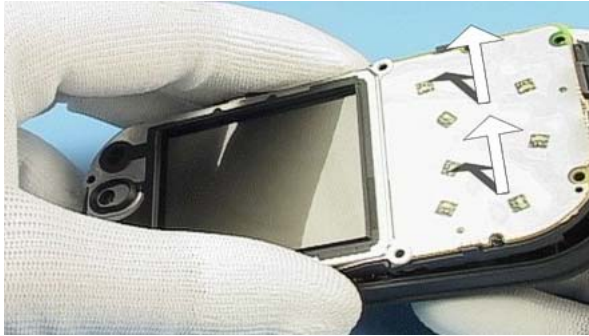
Separate the engine from the B-cover.
