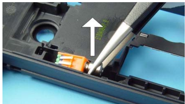
Remove the vibra motor.
